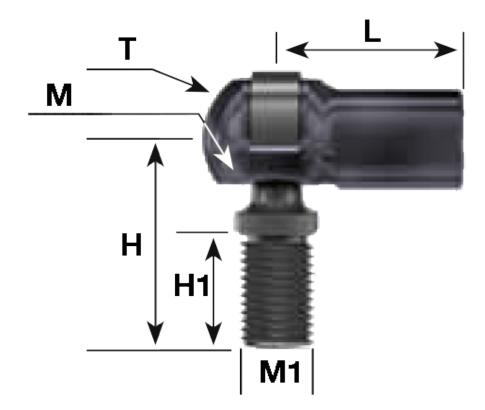
H = 29.3 H1 = 16.3 L = 25 M = Metal M1 = M10 T (Thickness) = Ø13
